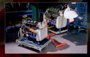
comparable characteristics to the Gen II three-cylinder engine. The four-cylinder engine comes in at about 118kg, which for an engine planned to produce 170-190hp, gives a significantly lower installed weight than equivalent avgas engines, along with the diesel's more frugal fuel burn. Typically three-cylinder units in RV-9s will average 15-16 litres per hour.
